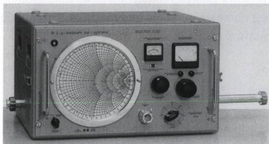
Fig. 10.1.1 The famous Z-g-Diagraph, a vector network analyzer family from Rohde & Schwarz that was manufactured from 1950 to 1977.
