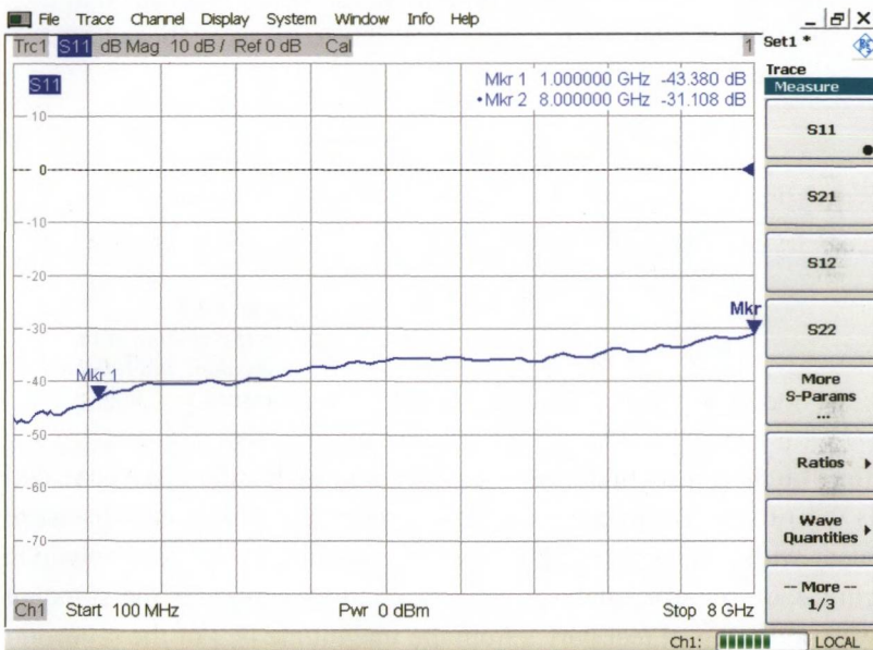
Fig. 4.3.3 Check of the match of a high-performance attenuator pad.
