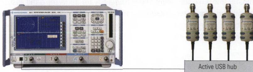
Fig. 7.1.10 R&S®ZVB4 network analyzer with four R&S®NRP-Z51 power sensors.
